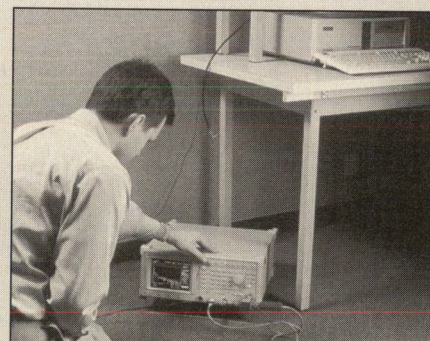
A technician uses the distance-to-fault mode to isolate the location of a poor (high SWR) connection in a high speed LAN.
