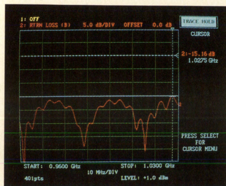
Figure 2: This swept frequency plot of a transmission line cable and antenna marginally meets the -15 dB return loss specification.
